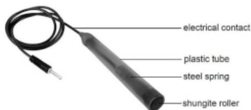
Fig. 1. Image of homemade solid-disk elite shungite electrode.
